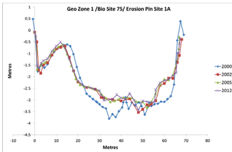
Figure 5.10. Surveyed cross-sections of erosion pin site 1A. Note vertical exaggeration.
