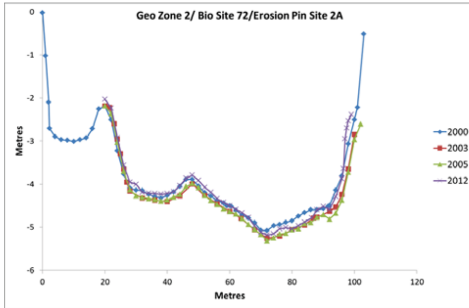
Figure 5.11. Surveyed cross-sections of erosion pin site 2A. Note vertical exaggeration.
