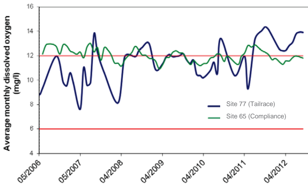
Figure 4.14: Average monthly dissolved oxygen levels at Gordon Power Station tailrace and Gordon above Denison (site 65) over the post-Basslink period.
