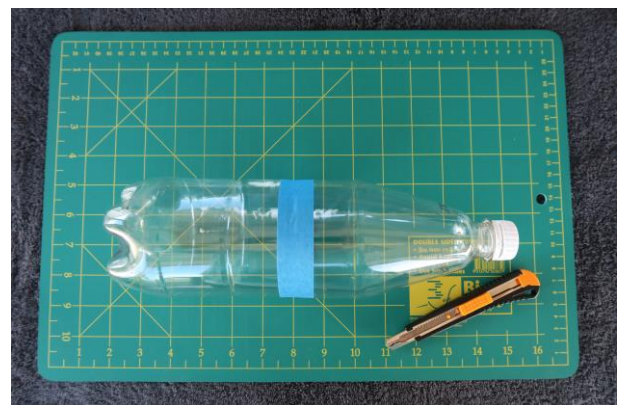
Figure 2: Step 2, cutting the bottle in half using masking tape
